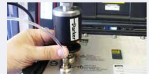
To remove the PRV, press down on the removal tool at the same time as lifting PRV off.
